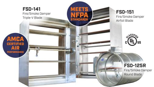
Pottorff's combination fire/smoke dampers bring together the fire barrier protection of a fire damper (preventing the spread of fire by closing upon the detection of high temperatures) and the smoke control of a smoke damper (limiting air leakage through ductwork, which is critical during a fire event) into one unit. Pottorff tests all of our combination fire/smoke dampers to UL's stringent requirements for fire resistance and leakage control.
